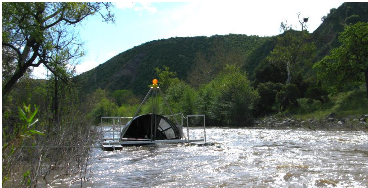
Figure 1. Rotary screw trap operating on the Arroyo Seco River (April 5, 2010).
